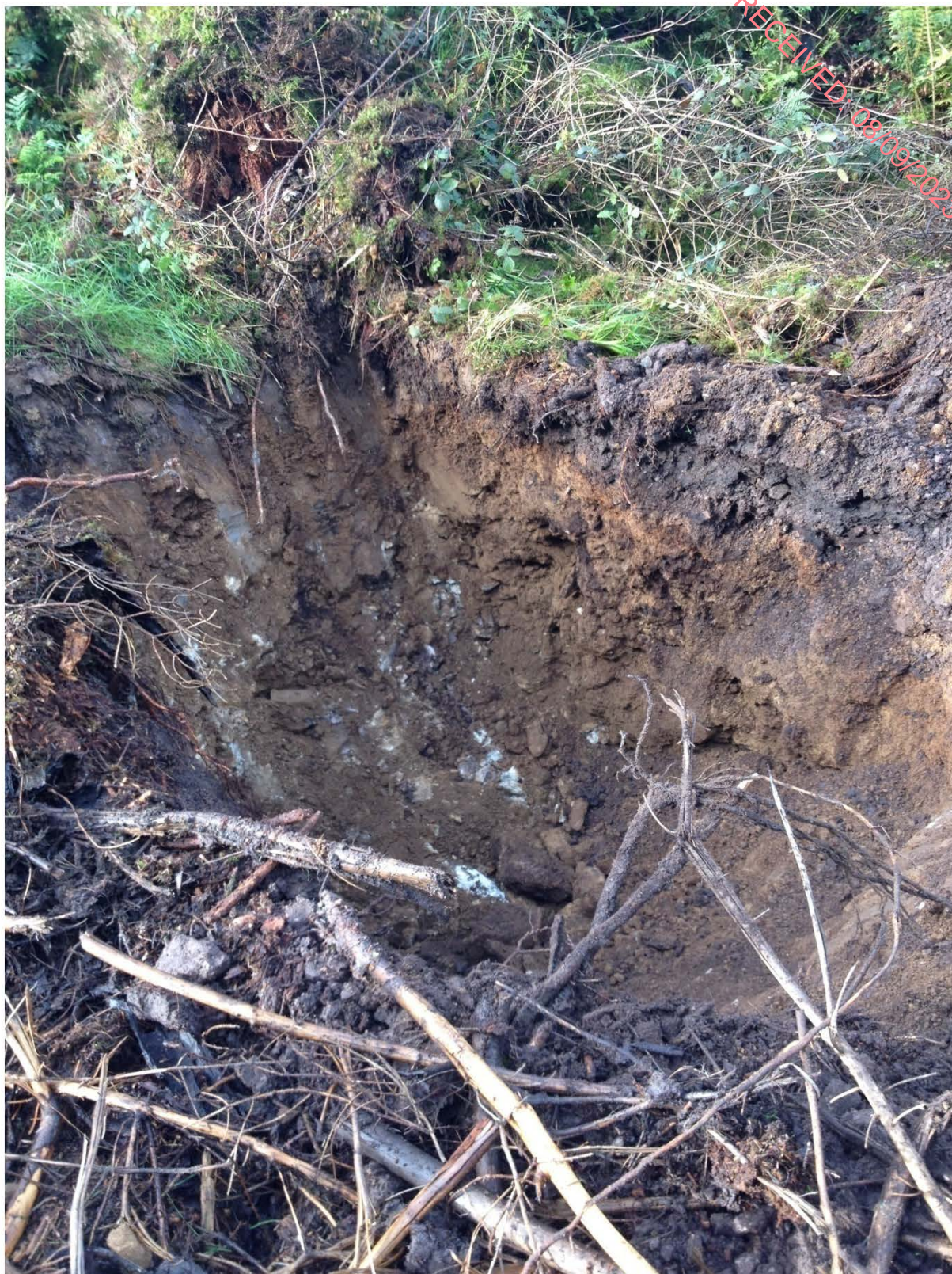
Trial pit at Borrow Pit 1
